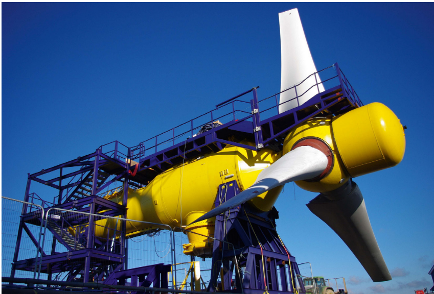
Figure 7: A tidal flow turbine being installed. (Courtesy of Alstom.)
